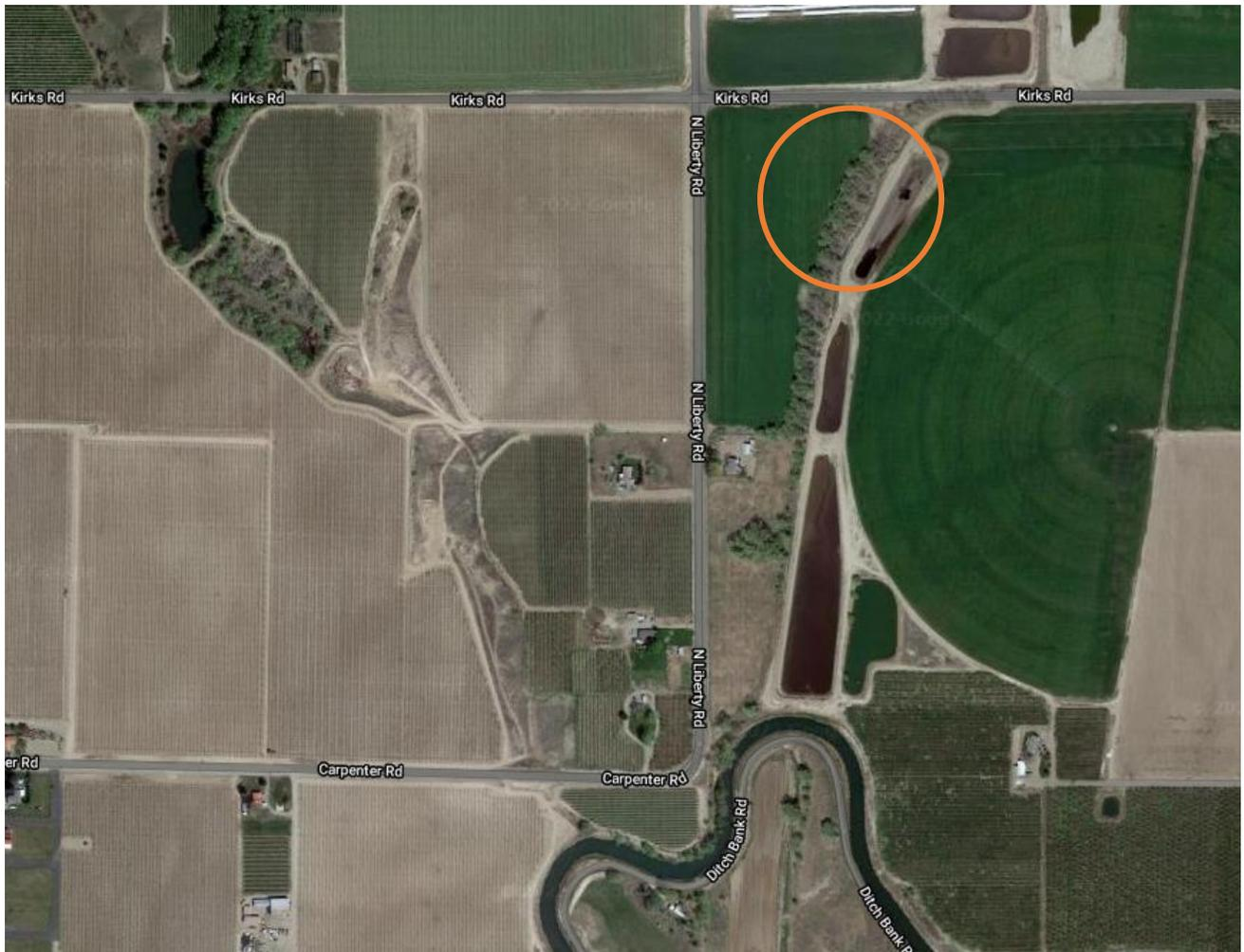
This 2.3 million gallon lagoon was built decades ago, apparently without a permit, in Yakima County where local regulation is minimal. It was constructed in a draw, next to an intermittent stream, and next to the Roza Irrigation Wasteway. Nitrate N levels in a nearby EPA monitoring well have exceeded 200 mg/L – twenty times higher than the safe drinking water standard of 10 mg/L. People and animals that drink water with 200 mg/L Nitrate N will get sick and often die.
